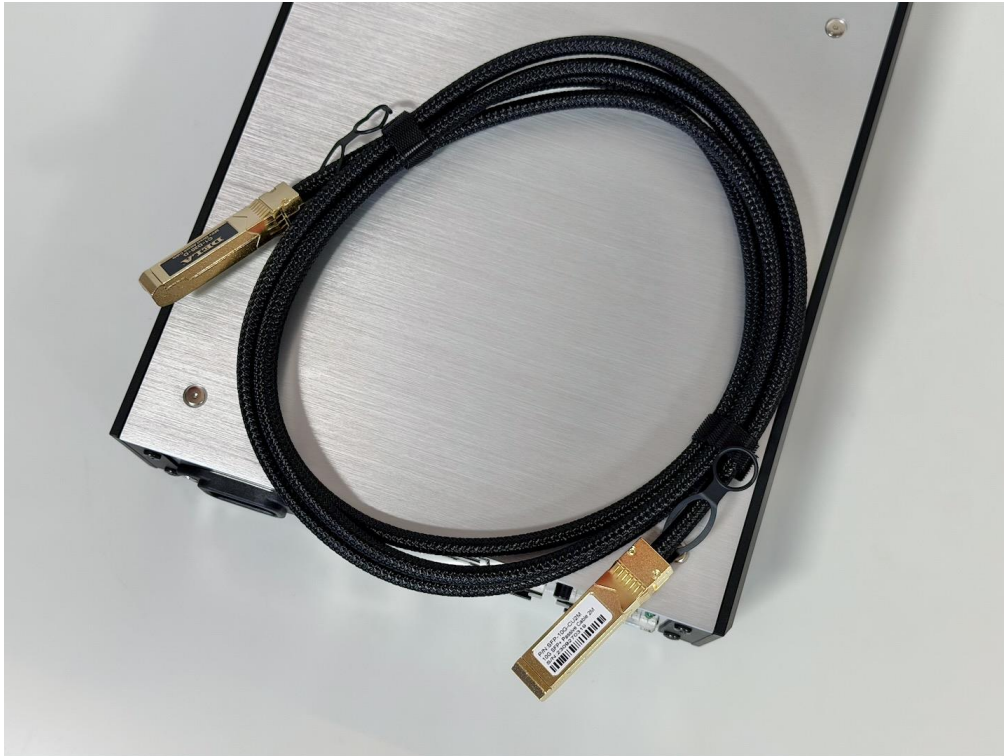
The electrical (non-optical) DELA C1 allows for a particularly direct connection to the data bus (Photo: F. Borowski)
