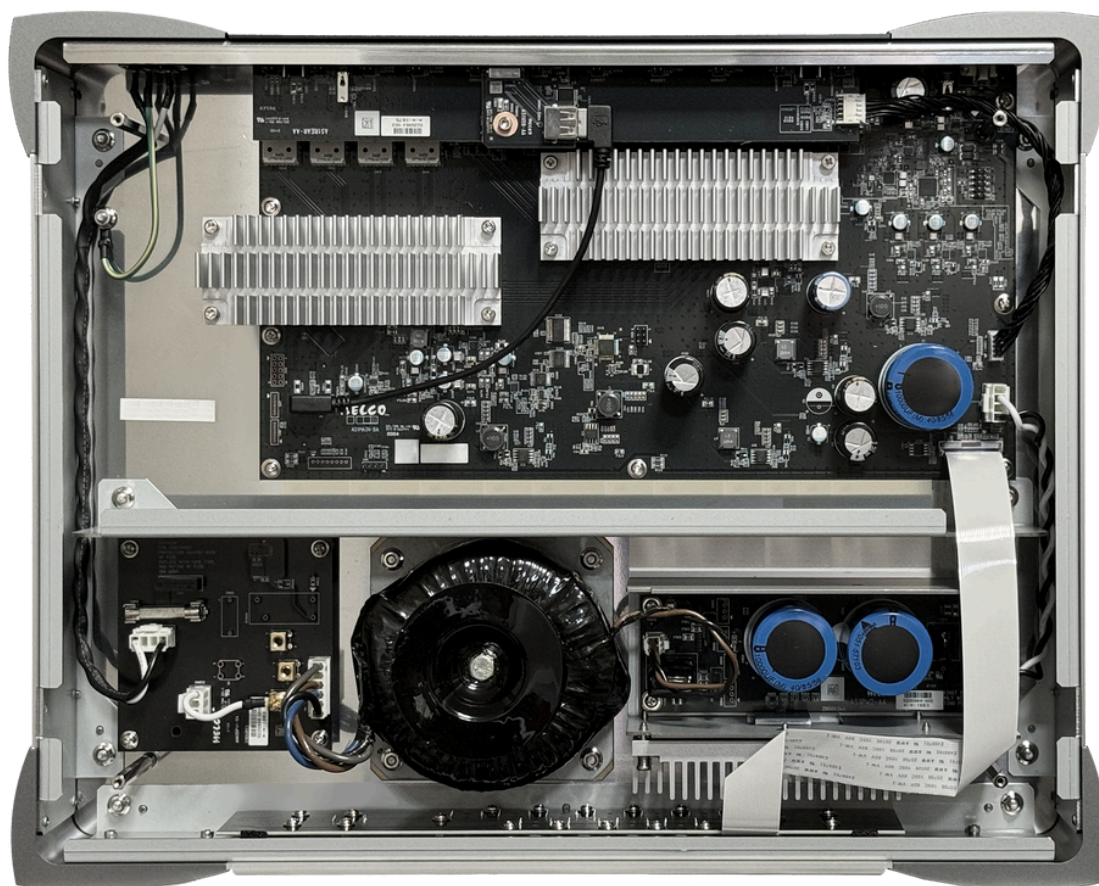
MELCO S1 Network Switch, internal layout
