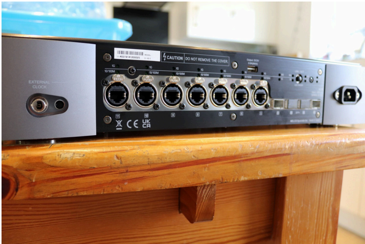
MELCO S1 Network Switch, rear detail with external clock BNC connection
